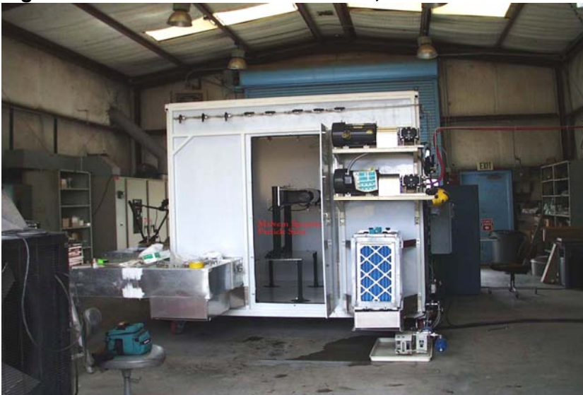
Figure 10 – An Aerosol Test Chamber, 14.5 m 3 total volume
